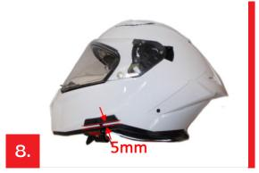
Fit the keypad on the left side (helmet on), approximately 5 mm from the lower edge of the shell using the provided adhesive. Make sure that there is full contact surface between the adhesive keypad and the outer shell.
