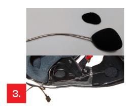
Place the microphone with wire on chin cover after applying the adhesive Velcro included in the package
