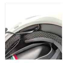
Place the BT controller in the designated slot on the back of the inner shell.
