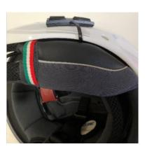
During the comfort cheekpads assembling, pass the flat cable of the remote control between the cheekpads's pp plate and the shell.
