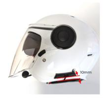
Fit the keypad on the left side (helmet on), approximately 10 mm from the lower edge of the shell using the provided adhesive. Make sure that there is full contact surface between the adhesive keypad and the outer shell.
